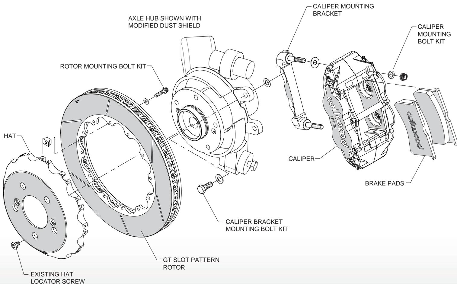
Figure 1. Typical Installation Diagram
